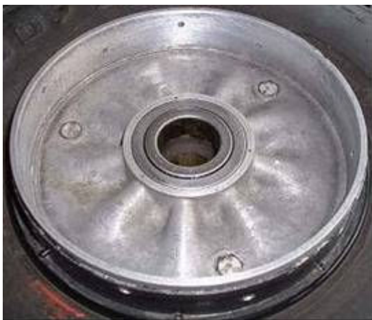
Figure 13 Cleaned-up lining housing
