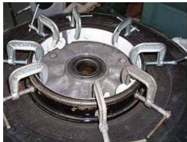
Figure 14 Clamping new lining using brake shoes.
