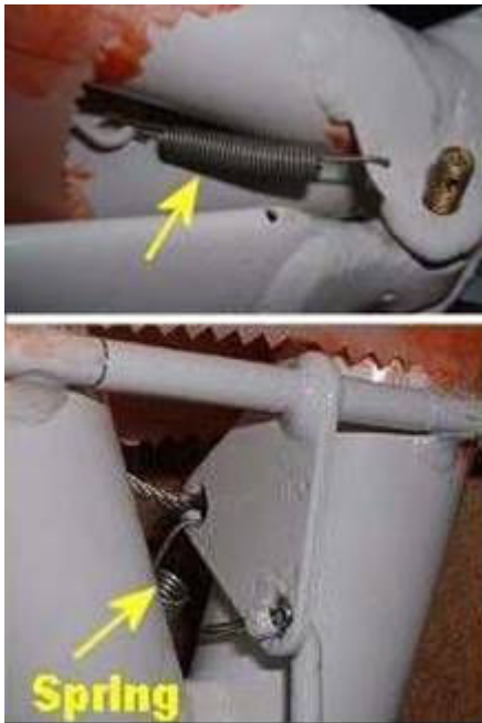
Figure 4 Two views of bellcrank spring
